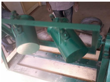
Fig5. Deval’s abrasion machine
