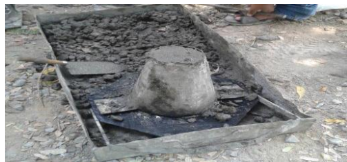
Fig.8. Slump test for conventional concrete
