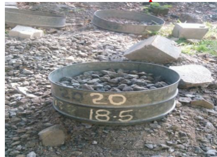
Fig4. Sieving of crushed concrete waste
