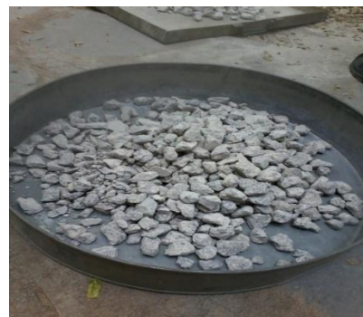
Fig6. Processed Recycled Aggregate
