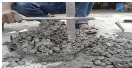
Fig.9. Slump of 10 % UPRA concrete
